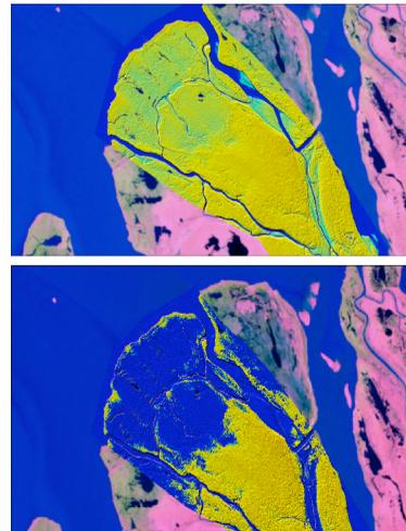
LIDAR survey to simulate effects of subsidence in the outer delta. Lower panel shows flooding to 1 m above MSL (upper panel). This could become the mean topography through a combination of regional and local subsidence.
