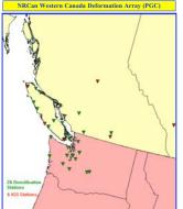
· From Herb Dragert, Pacific Geoscience Centre (PGC), NRCan Bernese GPS Software Version 4.2 · Double differenced observations 30 second data sampling · 10 deg elevation cut off · Fixed IGS precise orbits & ERP · Tropospheric zenith delay (every 2 hours) · Niell mapping function (dry) Tropospheric gradient (4/day) QIF ambiguity resolution
