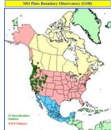
· From Scripps Institution of Oceanography (SIO) · GAMIT v9.72 software · Double differenced observation 2 minute data sampling for final solution · 10 deg elevation cut off · Fixed SIO precise orbits & ERP · Tropospheric zenith delay (random walk) Niell mapping function (dry & wet)
