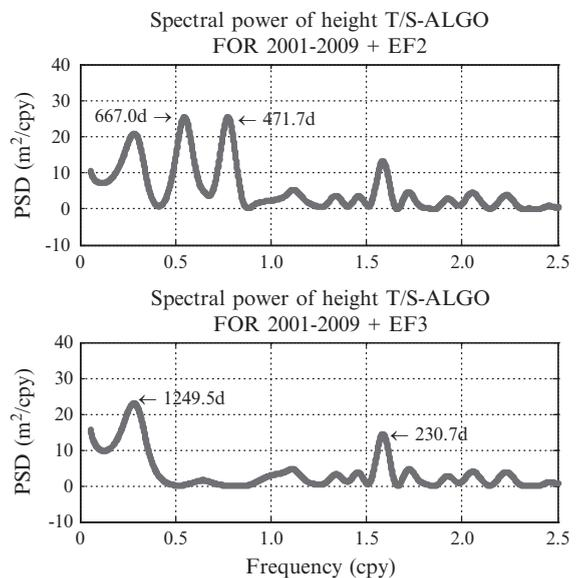
**Fig. 87.6** Power spectral density for station ALGO (Algonquin). *Top plot* is after enforcement of periods 1,904.5, 875.7 and 373.6 days. *Bottom plot* is after enforcement of periods 1,904.5, 875.7, 373.6, 667.0 and 471.8 days
