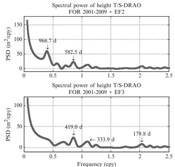
**Fig. 87.10** Power spectral density for station DRAO (Penticton). *Top plot* is after enforcement of periods 1,388.9 and 361.7 days. *Bottom plot* is after enforcement of periods 966.7 and 582.5 days
