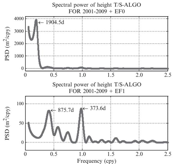
**Fig. 87.5** Power spectral density for station ALGO. *Top plot* is with no periods enforced. The *bottom plot* is after enforcement of period 1,904.5 day
