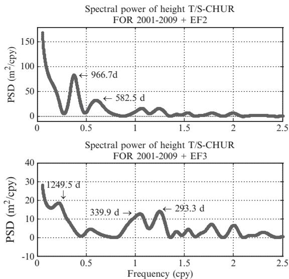
**Fig. 87.8** Power spectral density for station CHUR (Churchill). *Top plot* is after enforcement of periods 1,760.5, 475.2 and 374.0 days. *Bottom plot* is after enforcement of periods 1,760.5, 475.2, 374.0, 966.7 and 582.5 days
