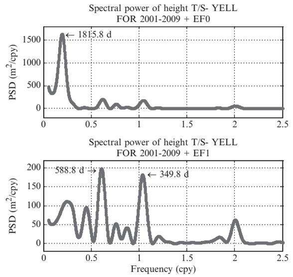
**Fig. 87.13** Power spectral density for station YELL. *Top plot* is with no periods enforced. *Bottom plot* is after enforcement of period 1,815.8 day
