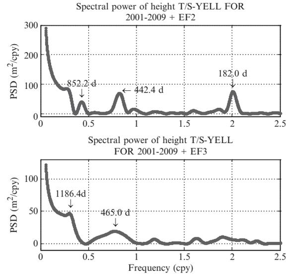
**Fig. 87.14** Power spectral density versus frequency for station YELL. *Top plot* is after enforcement of periods 1,815.9, 588.8 and 349.8 days. *Bottom plot* is after enforcement of periods 1,815.85, 588.79, 349.831, 852.2, 442.4 and 182.0 days
