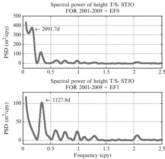
**Fig. 87.11** Power spectral density for station STJO. *Top plot* is with no periods enforced. *Bottom plot* is after enforcement of period 2,091.7 days
