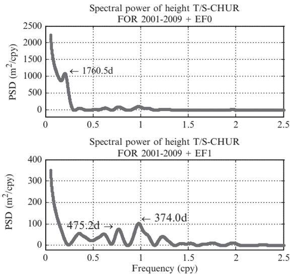
**Fig. 87.7** Power spectral density for station CHUR. *Top plot* is with no periods enforced. *Bottom plot* is after enforcement of period 1,760.5 day
