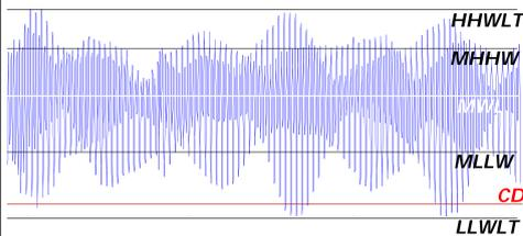
Chart Datum (CD) is the vertical datum for nautical charts. In Canada, CD targets Lower Low Water Large Tide (LLWLT), the lowest predicted tide in a 19-year astronomical cycle (see figure). It rarely coincides with LLWLT, however, especially where CD was set tens of years ago and where relative sea level rise is large. In this figure we show 4 tidal levels, but many more can be defined. We currently have HyVSEPs for CD, 6 high and low tidal levels, and Mean Water Level.
