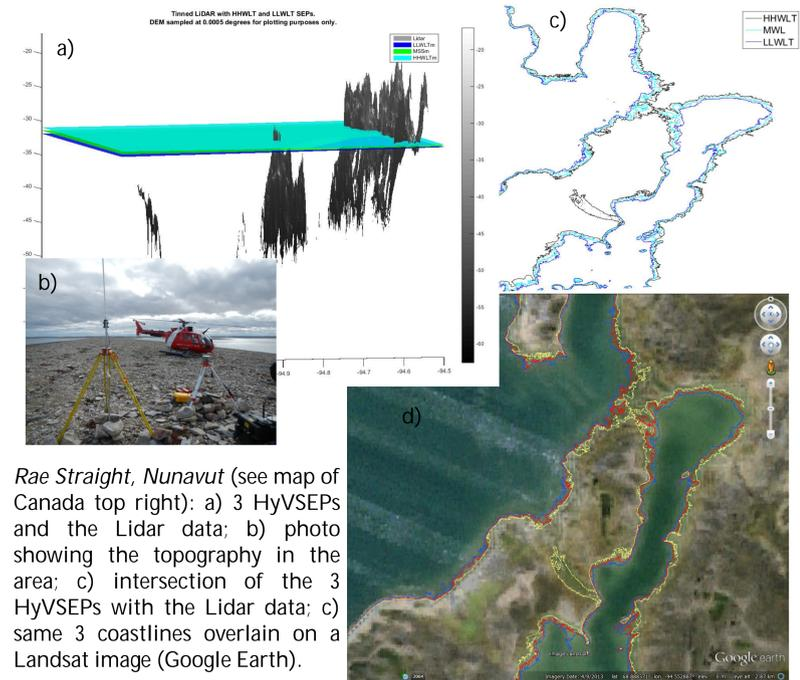
Rae Straight, Nunavut (see map of Canada top right): a) 3 HyVSEPs and the Lidar data; b) photo showing the topography in the area; c) intersection of the 3 HyVSEPs with the Lidar data; d) same 3 coastlines overlain on a Landsat image (Google Earth).
