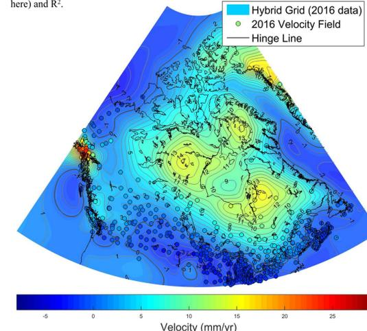
Figure 6. Hybrid grid calculated as in Fig. 5 but including the 2016 data. Differences between the two grids are due to denser data in northern BC and Alaska (defining the Little Ice Age uplift), and new data from the north central states. New 2017 data in Nunavut is likely to adjust the uplift dome west of Hudson's Bay. The 2016 GPS solutions have not yet been manually quality controlled.
