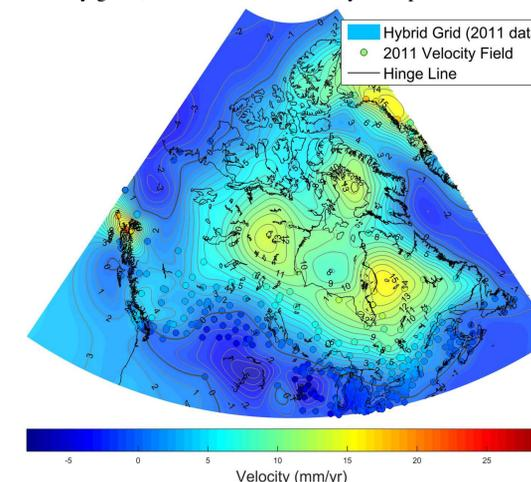
Figure 5. Hybrid grid calculated using the procedure described in Section 3, using the 2011 data used for NAD83v6vg, and the Laur16Innu+elastic combined models. Comparison with Figure 2 highlights the effect of changing the interpolation method and including the geophysical models.
