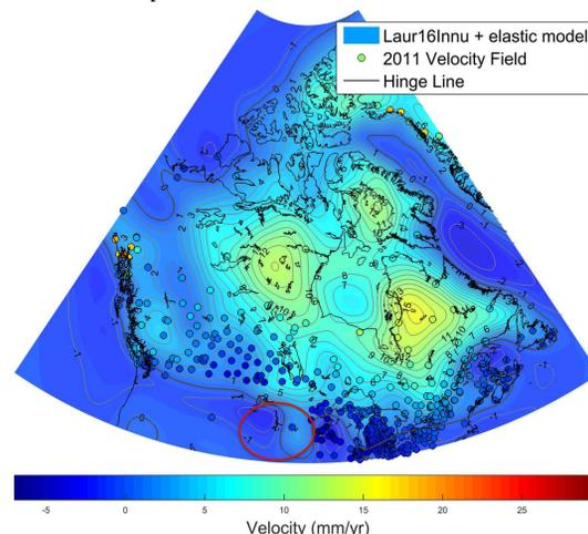
Figure 4. Combination of the Laur16Innu GIA model<sup>1</sup> and the elastic model. Laur16Innu is derived from the ICE-5G ice history model, adjusted to optimize the fit in 4 regions of northern Canada. The feature circled in red is from the Ice-5G model, and does not appear in ICE-6G<sup>2</sup>. We also tested NAICE<sup>3</sup>.
