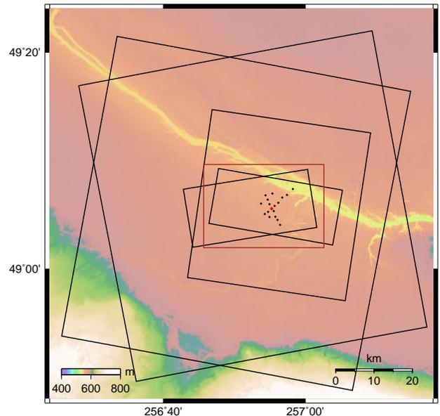
Fig. 1. Area of interest is outlined in brown, RADARSAT-2 frames used in this study are outlined in black: large frames are from ascending and descending Wide Ultra-Fine (U7W2), smallest frames are from ascending Spotlight (SLA18) and descending Spotlight (SLA12) and remaining frame is from descending Fine Quad-Pol (FQ28) beams. Digital Elevation Model is plotted in background. Black diamonds mark locations of observation sites and red diamond marks location of injection well.
