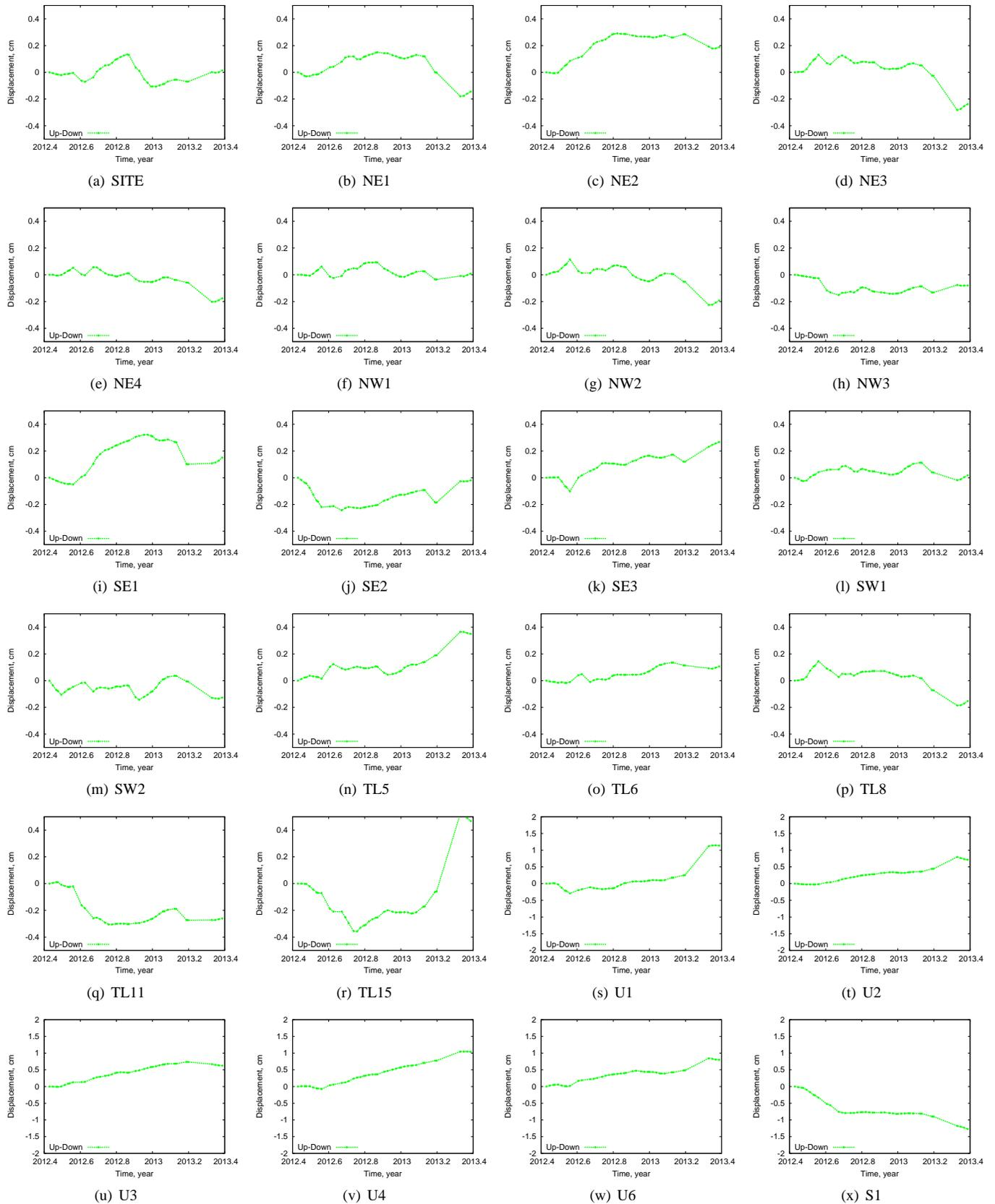
Fig. 2. Time series of vertical deformation. Points NE, NW, SE and SW correspond to approximate locations of observation sites and point SITE corresponds to location of injection well. Points U1-U5 experience faster than normal uplift and point S1 experiences faster than normal subsidence. Note change in scale for U1-U5 and S1 points.
