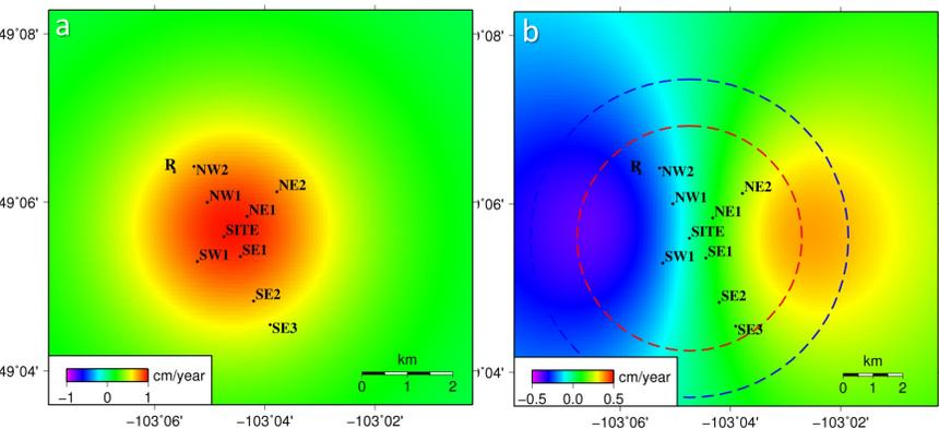
Modeled vertical (c) and horizontal (East-West) (d) deformation rates superimposed on observed MSBAS deformation rates. Presented here signal is expected in case of CO<sub>2</sub> injection. Monitoring sites and reference region "R" are plotted in black. In (d) red circle marks region where horizontal displacements produced by injection reach maximum. Blue circle marks region at which vertical and horizontal displacements produced by injection are equal.
