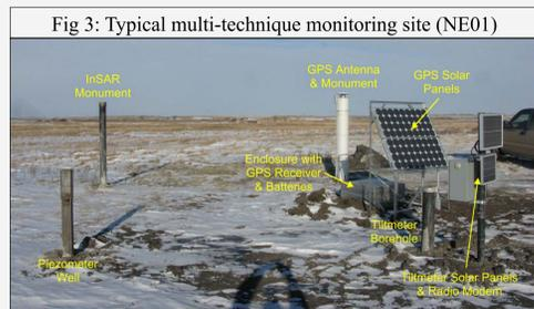
Fig 3: Typical multi-technique monitoring site (NE01)
