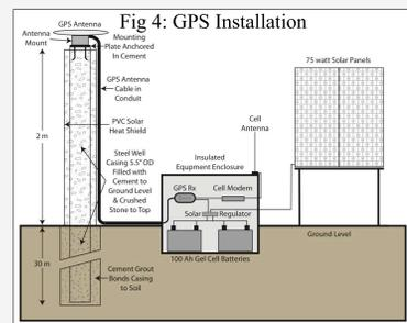
Fig 4: GPS Installation
